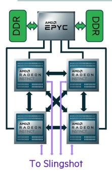
2560 nodes with 4 x MI250X + 1 x AMD Trento processor, 512 GB host memory and 512 GB device memory (HBM2) 4 x 200 Gbit/s NIC Infinity Fabric
