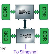
2x 64-core AMD Milan processors per node 1376 nodes with 256 GB, 128 with 512 GB and 32 with 1TB 1 x 200 Gbit/s NIC
